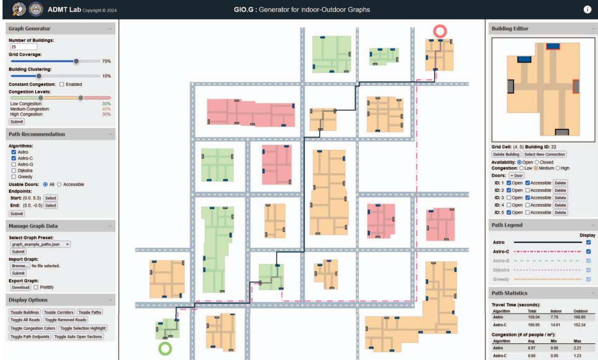
Fig. 3: The front-end Web Interface prototype for GIO.G
