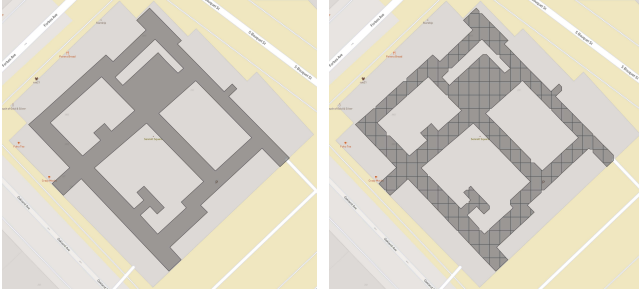
Figure 3: Floor plan of the Sennot Square building at the University of Pittsburgh campus (left) converted to a Building Grid Layout (right).
